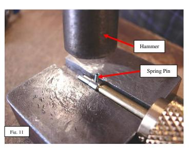
A-11. Push the "o-ring" into the "clevis" by inserting the "shaft assembly" into it. Push the parts together and align the hold on the "clevis" with the hole on the "shaft". Using a hammer, install the small "spring pin" into the hole. Use a "punch" to be sure the "pin" is fully inserted into the assembly.
