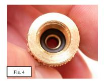
A-4. Push the "o-ring" down towards the "gold washer" till it fits in the groove inside the "nut". This "o-ring" should hold the other parts in place.
