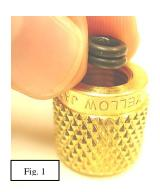
A-1. Place the two medium sized" o-rings" inside the "nut". The O-rings need to be stacked and seated flat on the bottom of the "nut".
