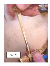
B3. Place "valve opener" into the "side port of ball valve" (gold end first). Use the "tightening tool" shown to screw in the "valve opener". Do not over tighten.
