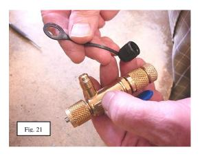
B4. Place the "cap strap" onto the "side port of the ball valve" as shown.
