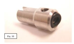
A-10. Place the "o-ring" inside the "clevis" as shown.
