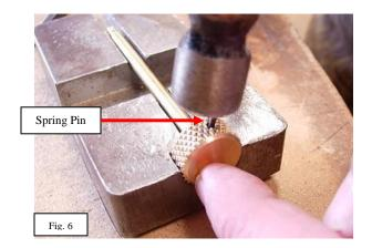
A-6. Rotate the "knob" until the larger hole is facing up, and twist the shaft until the holes of both parts are aligned. Install the longer "spring pin" into the shaft assembly using a hammer. Use a "punch" to ensure the "spring pin" is recessed into the "knob".
