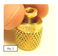
A-2. Place the "washer" on top of the two o-rings. This also needs to sit flat on top of the orings.
