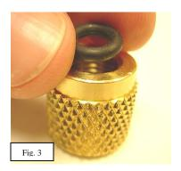
A-3. Install the "large o-ring" into the "nut". The "o-ring" should sit on top of the "gold washer".
